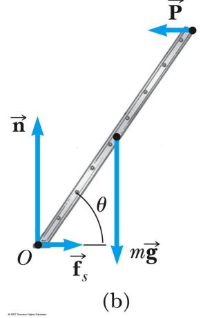
A 800N-man is climbing a uniform ladder that is 5m long and weighs 180 N. The ladder makes an angle of 53.1°. Find the normal and friction forces on the base of the ladder.
