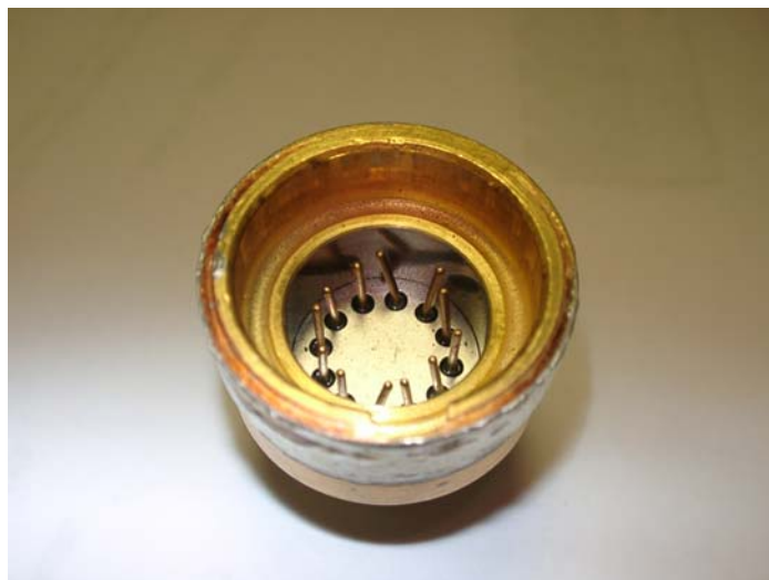
Example of damage pins removed from a sample chamber.
