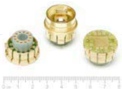
► Specialized pucks, 2.4 cm in diameter, are used for different measurement applications.
