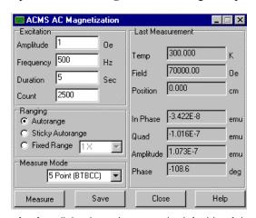
Figure 4-5. **AC Magnetization** dialog box. Items on the left side of the dialog box designate measurement conditions that should be set prior to initiating the measurement. Items on the right side of the dialog box display the results of the last immediate-mode AC measurement.
