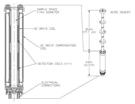
Figure 1-1. ACMS Insert and Coil Set
