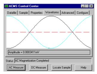
Figure 4-6. Example of plot of AC measurement in **Waveforms** tab. The light blue line that may appear in the tab is the waveform reference and indicates the ideal measurement results. You use the waveform reference to help determine the effectiveness of the measurement. The waveform reference is not visible if the measured waveform and ideal plot are nearly identical.
