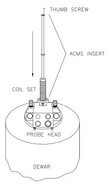
Figure 2-1. Installing the ACMS Insert
