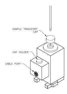
Figure 3-3. Installing the Sample
