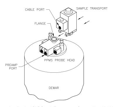
Figure 2-2. Installing the ACMS Sample Transport on a System without High Vacuum
