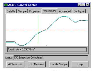
Figure 4-13. Example of plot of DC measurement in **Waveforms** tab. The light blue line that may appear in the tab is the waveform reference and indicates the ideal measurement results. You use the waveform reference to help determine the effectiveness of the measurement. The waveform reference is not visible if the measured waveform and ideal plot are nearly identical.
