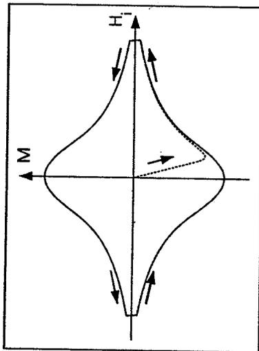
Figure 7: Sketch of a complete magnetization hysteresis loop versus internal magnetic field  $H_i$ . The dashed line is the initial response following zero field cooling, while the solid line is the response for repeated cycles between maximum and minimum field strengths. The arrows indicate the direction of the field sweep, and the hysteresis is the difference in magnetization at a given field during increasing and decreasing field sweeps.
