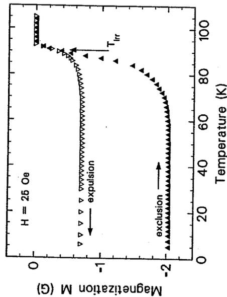
Figure 4: Flux exclusion (shielding) versus increasing temperature (solid triangles) and flux expulsion (Meissner effect) versus decreasing temperature (open triangles) in a 25 Oe external field for a superconducting  $\text{YBa}_2\text{Cu}_3\text{O}_{7-\delta}$  single crystal. Exclusion and expulsion are equal for temperatures above the irreversibility point  $T_{\text{irr}}$  ( $\approx 90.5 \text{ K}$  at 25 Oe);  $T_c$  is 92 K.
