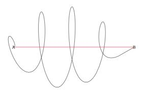
FIG. 20: Path-independence of the work done by a force. For any force the work is given by eq. (27), but for special "conservative" forces, the work does not depend on the actual path which connects points A and B. For such forces one can talk about potential energy,  $U(\vec{r})$  and use eq. (28) to determine the work on a path. The electrostatic force is of that kind.
