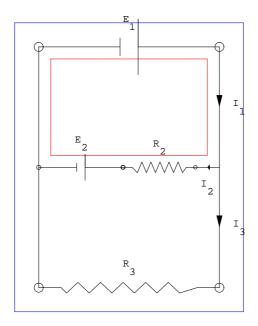
FIG. 32: Example of a two-loop circuit
