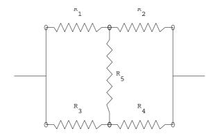
FIG. 29: Irreducible circuit
