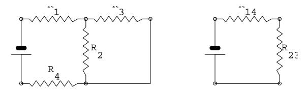
FIG. 28: Example of the reduction method
