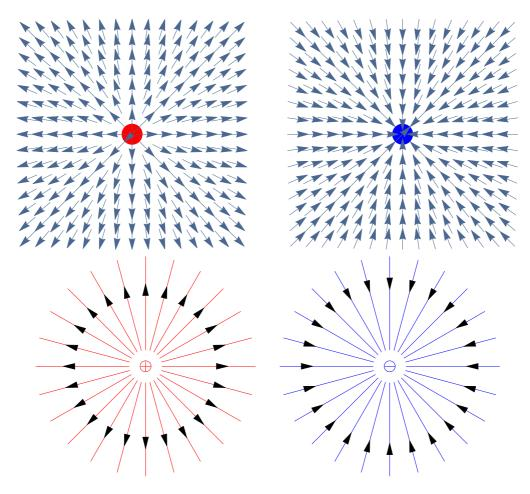
FIG. 9: Vector fields (upper row) and electric field lines (lower row) due to single point charges. Note that the field becomes infinitely strong when a charge is approached.
