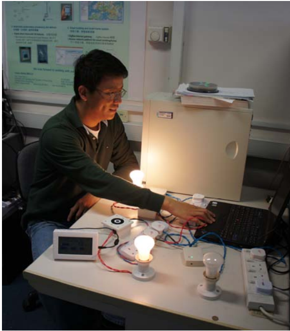
Figure 3-10 Testing the controllers and Control Logic for Smart Grid by Dr. Guanghai Yang
