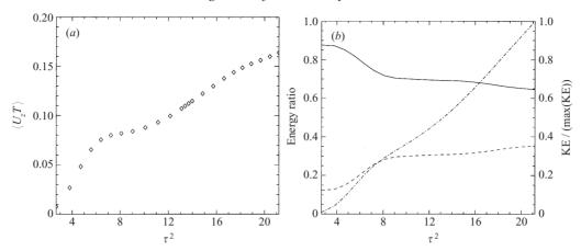
FIGURE 18. (a) Volume-averaged advective fluxes as a function of time. (b) Partition of kinetic energy as functions of time; the solid line is the partition of the kinetic energy in the vertical direction and the dashed line is along the horizontal directions; the dash-dotted line is the normalized kinetic energy.
