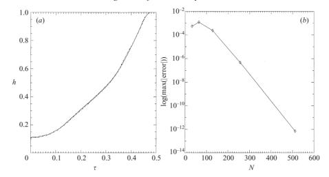
FIGURE 1. (a) Comparison between the spectral-element code (solid line) and the spectral code (dashed line) for simulation of a single-mode perturbation at the interface. Plotted is the mixing zone width h as a function of time  $\tau$ . (b) The spectral code shows exponential convergence for a fixed interface thickness of 0.15 in the single-mode simulation. The error is defined as the deviation from the simulation with a resolution of 1024.
