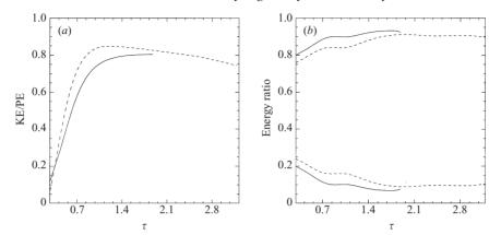
FIGURE 26. (a) Ratio of total kinetic energy to total potential energy available in the system as a function of  $\tau$ . (b) Vertical partition of the total kinetic energy and horizontal partition of the kinetic energy as functions of  $\tau$ . In both panels, we plot two-dimensional (dashed lines) together with three-dimensional simulations (solid lines).
