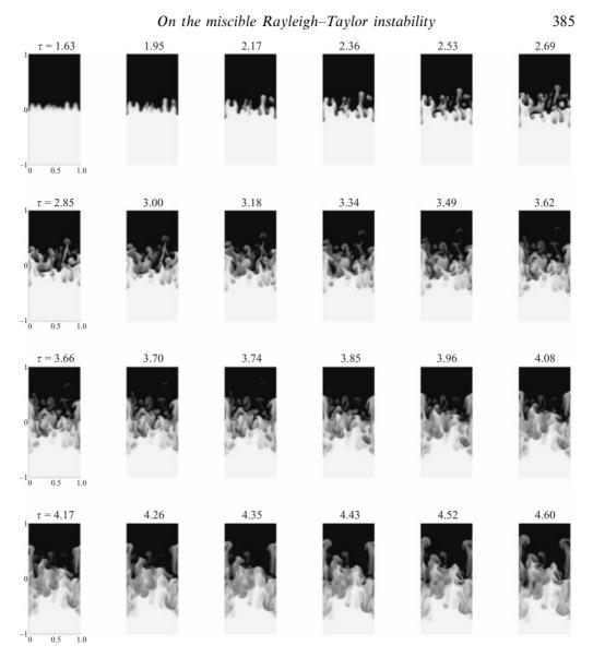
FIGURE 4. Time series of the temperature from the three-dimensional simulations. The slices (T(x, y = 0, z)) are taken at the same times as those for the corresponding two-dimensional frames (figure 3).
