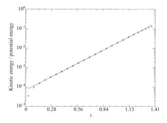
FIGURE 9. Early evolution of the three-dimensional random perturbation. The diamonds are data from the numerical simulation. The solid line is the best fit on the log-linear plot (for  $0.28 \le \tau \le 1.13$ ), and the duration of the linear growth is about 4 e-folding times with a growth rate of 8. The growth rate obtained from the analytic results ( $n^2 = gAk$ , with gA = 10 and  $k \sim 8$  from the power spectrum of our initial perturbation at the interface), is 9.
